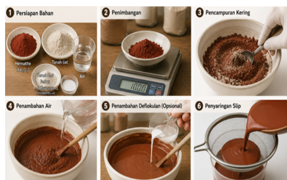
Gambar 3. Proses persiapan slip-clay-hematite
