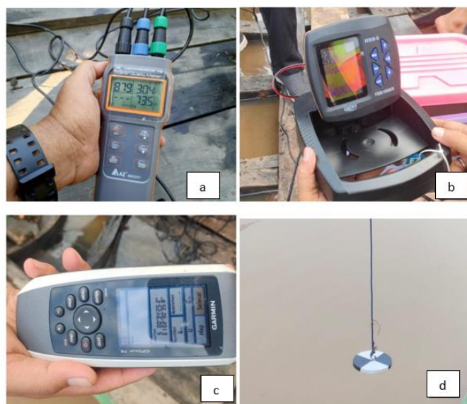
Figure 2. Fish Survey Supporting Equipment, a) Water Quality Meter AZ86031, b) Fish Finder Lucky FF918, c) Garmin GPS, d) Sacchi Disk Data Analysis
