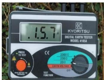
Gambar 2. Digital Earth Tester Kyoritsu model 4105A
