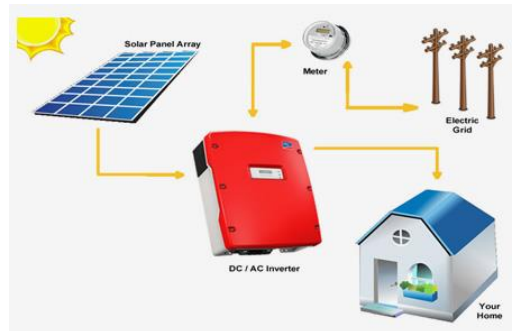
Gambar 1.1 Skema Sistem PLTS On Grid (Ramadhana, dkk, 2022)
