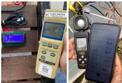
Gambar 5. Proses Kalibrasi Sensor BH1750
