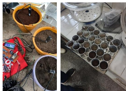
Gambar 4. Proses Kalibrasi Sensor Soil Moisture SEN0308
